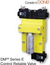
The valve also provides feedback to the control system about the valve's condition via a pressure switch. The switch isn't part of the safety system inherent in the valve; it's used for diagnostics. An abnormal valve operation, or fault, occurs when the two internal elements don't synchronously shift within 100ms of each other. This helps monitor for a sticky or sluggish valve, meeting "diminished performance" requirements of the ANSI/PMMI B155.1 standard.
